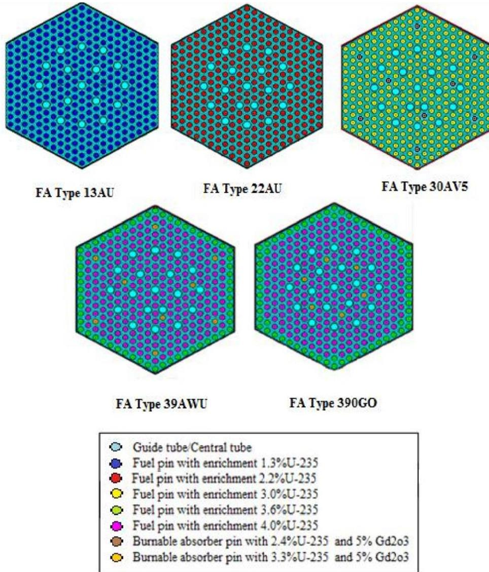
**Figure 2.** Pin layout of the FA types 13AU, 22AU, 30AV5 and 39AWU and features; one of those is to
