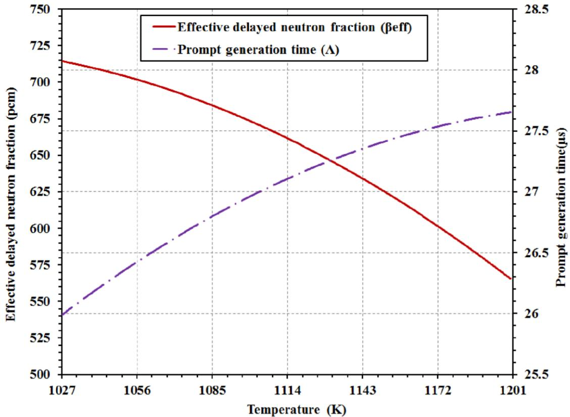
**Figure 6.** Variations in kinetic parameters versus temperature rising
