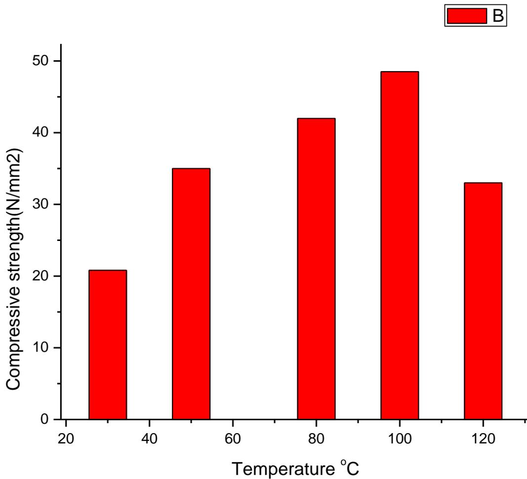
**Fig1. Effect of temperatures on the compressive strength of Mix3**
